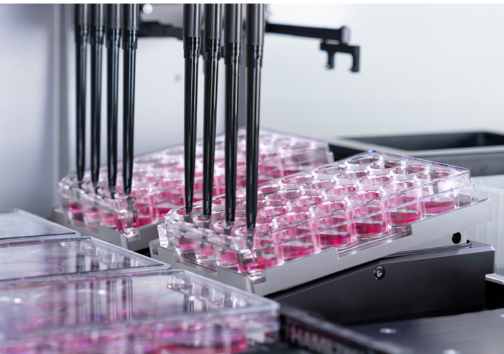
The tilted position provides precise liquid handling without disturbing adherent cells.
